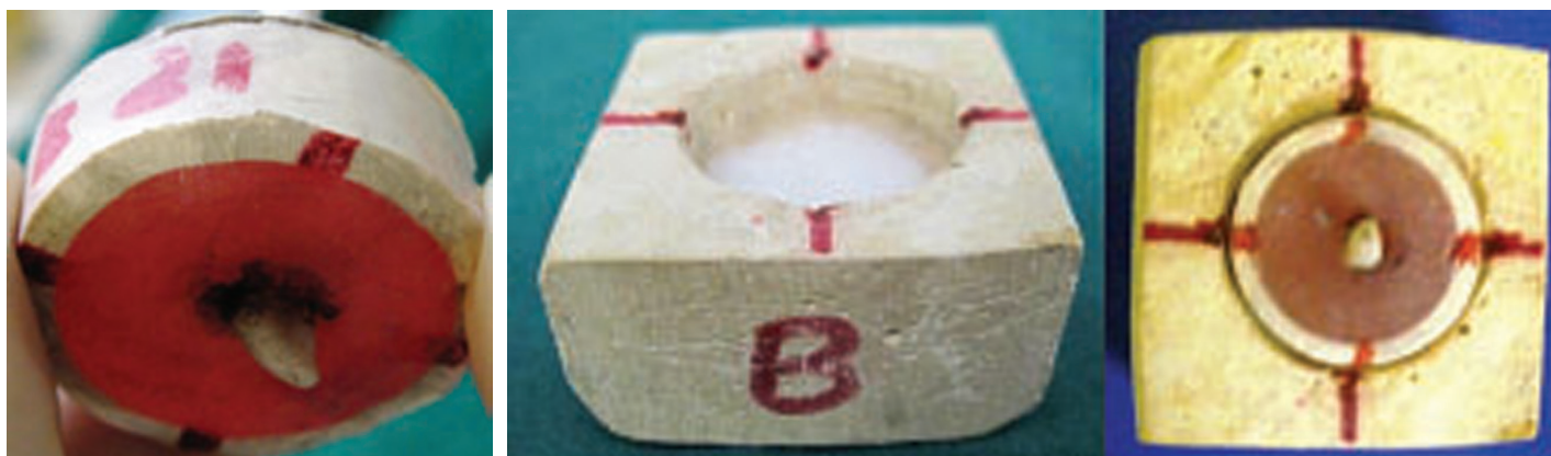
[Table/Fig-1]: Specimen after periodontal ligament simulation with apex exposed for recording images. [Table/Fig-2]: Customised jig for placement of specimens under stereomicroscope.
